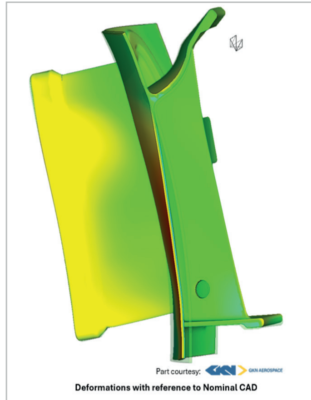
Figure 1: Deviation during simulation with reference to nominal CAD
